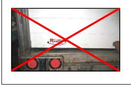
Door is not level – high on one side. To correct: Close the door and gently loosen the cable drum on the high side until the door is level. Re-tighten the fasteners securely.
