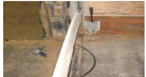
**Step 8** Bend out a small section of track, on one side, 12" above the top of the panels being replaced.
